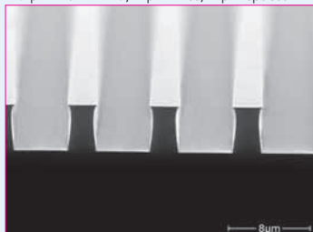
4 µm ma-P 1240, 3 µm lines, 5 µm spaces
