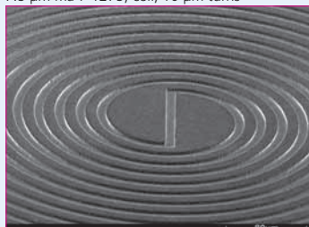
5 µm electroplated Ni coil, 10 µm turns
