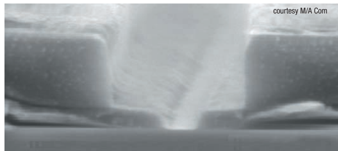
100nm gate profile imaged in 495K PMMA with 8.5 MAA Copolymer on top.
