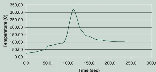
The typical profile above is designed for use with high-Pb (lead content 80% or greater) alloy in a forming gas or nitrogen atmosphere (100 ppm oxygen or less). It can serve as a general guideline for establishing a profile for your process and should be regarded as a typical example. Adjustments to this profile may be necessary based on assembly size, thermal density, and other factors. Use of other alloys with lower or higher liquidus temperatures will also require changes.
